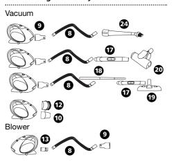
Note Make sure the correct end is fixed to the blower adapter, (smooth end).
